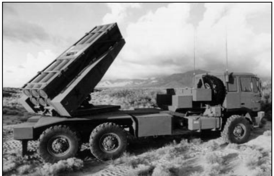
This is a promotional photograph of a HIMARS vehicle with a six-pack container of Multiple Launch Rocket System rockets on the launcher.
