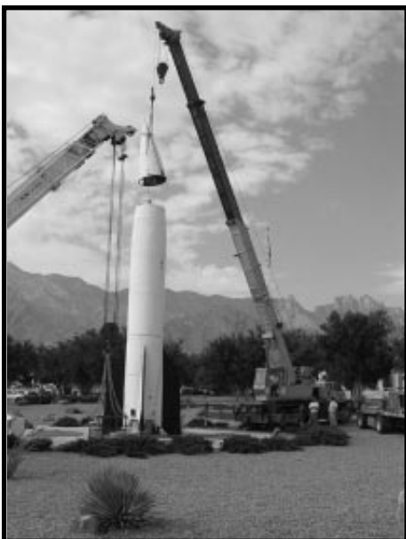
The V-2 warhead and guidance section are gently lifted off.
