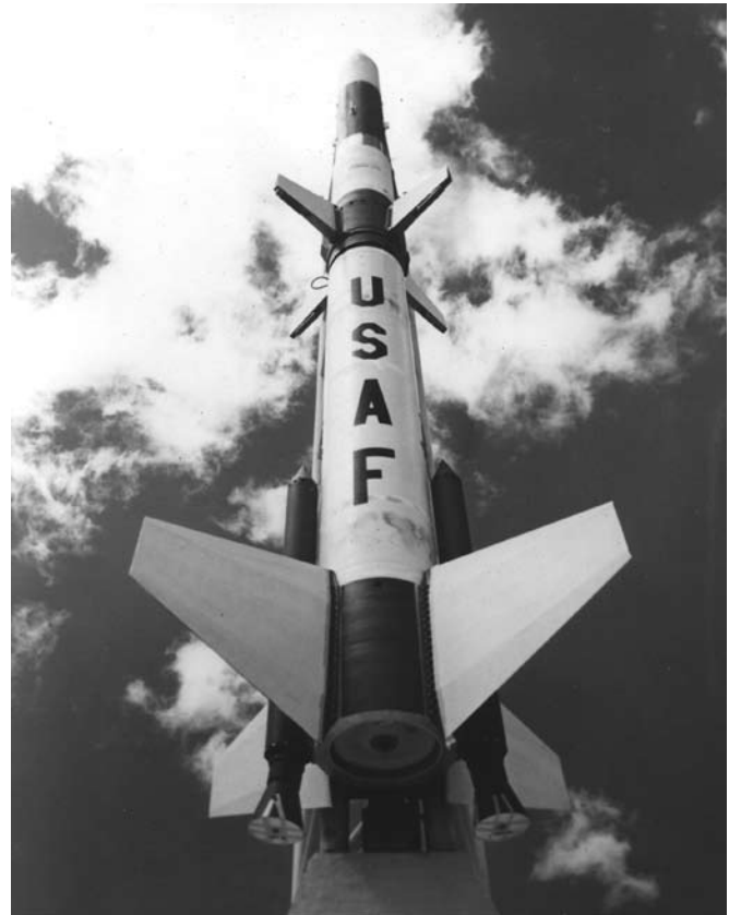
The Air Force Athena Missile sits on its rail ready to launch from Green River, Utah.
