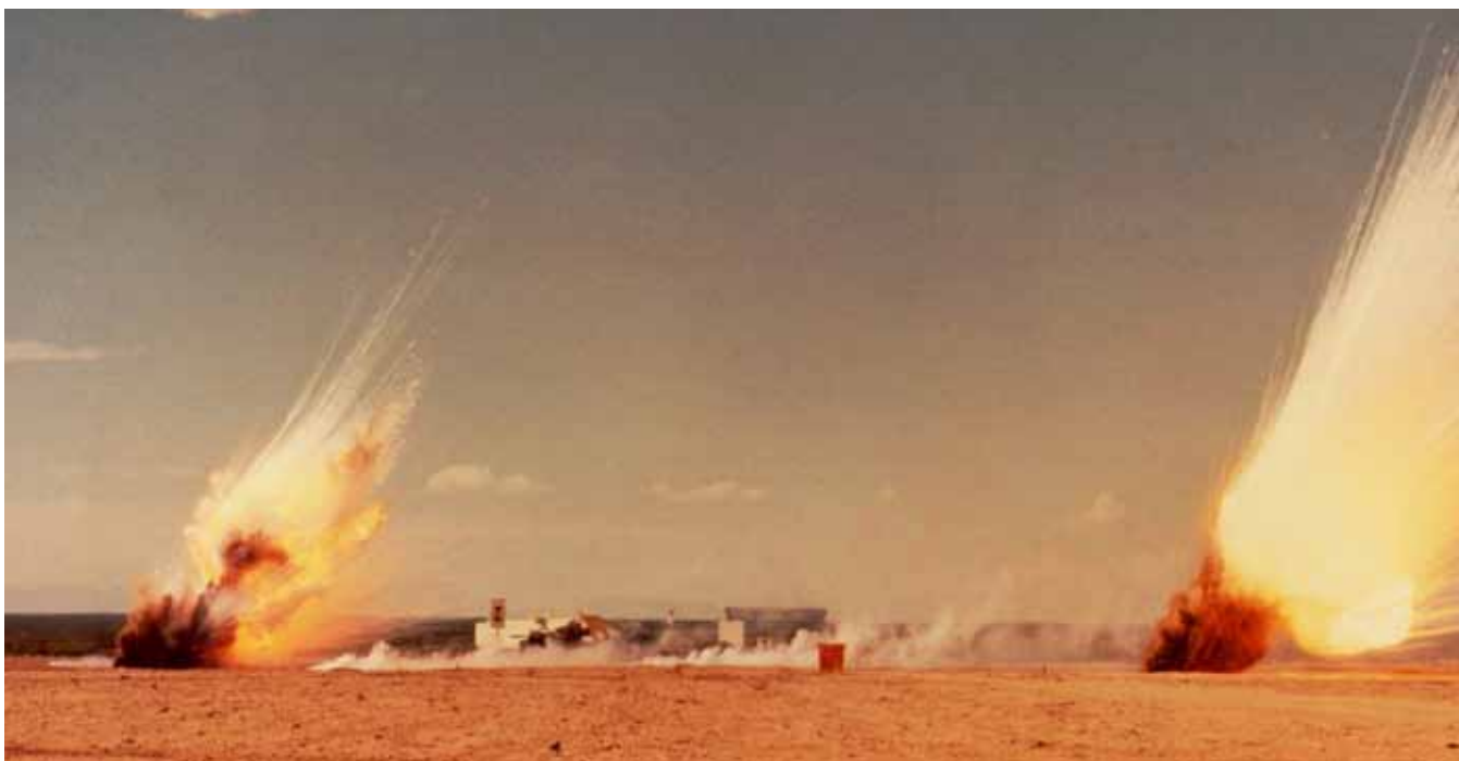
A typically spectacular White Sands photo of static artillery rounds being exploded in the test area to generate the dust needed for the DIRT 1 testing. Photo courtesy of Bruce Kennedy
