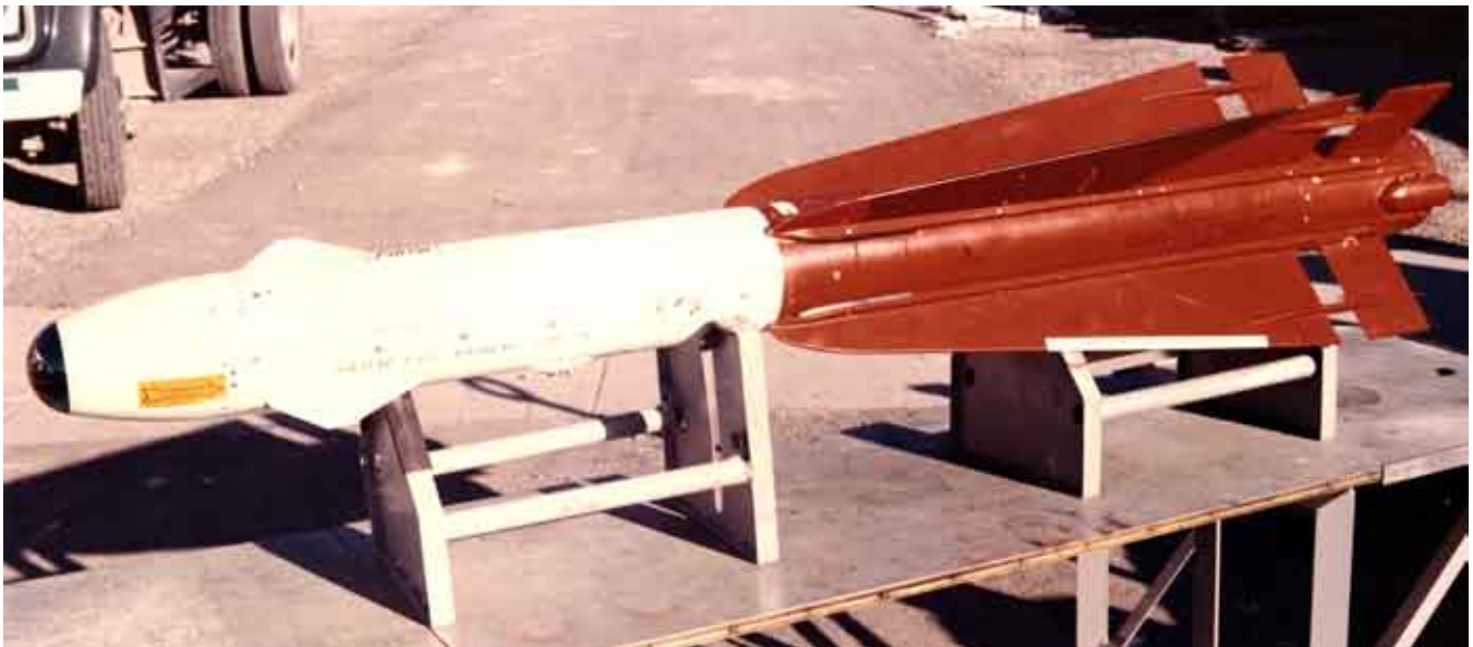
This color image of a Falcon is from the WSMR Museum Archive. Caption information indicates this is a "GAR-2B" version of the missile. That means it is an AIM-4 Falcon equipped with an infrared seeker. This was the last operational version of the Falcon.
