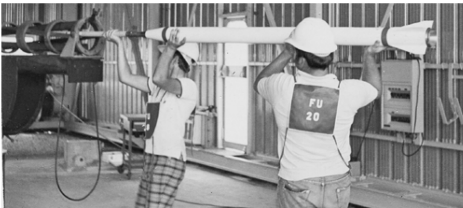
A Super Loki being loaded into a launcher. Hard to believe this small rocket could carry a payload to 50 miles above the ground.
