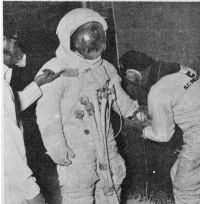
David Burris after his third session in the WSMR dust chamber. Technicians checked the suit's joints and fabric after each 30-minute period in the test room.
