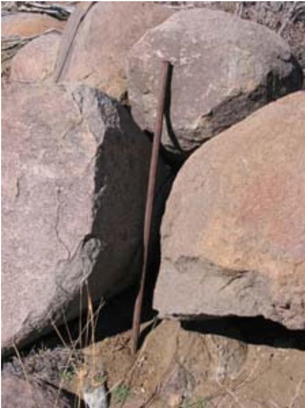
A rock drill. One person would hold the drill while another hit it repeatedly with a sledge hammer. Very slowly the team would drill holes into solid rock. Once deep enough the holes would be filled with dynamite and exploded to make a larger hole in the rock. (Photo by Jim Eckles)
